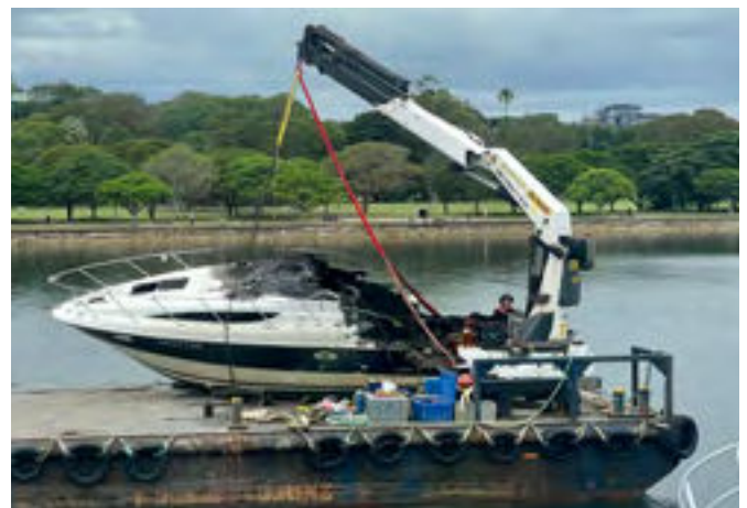
Fig 14: Fire damaged vessel as a result of refuelling accident.
